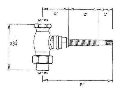
If solder/brazing the fitting connections, pre-assemble adapter fitting to copper piping. Use Teflon tape or equivalent to seal the threaded joints.
